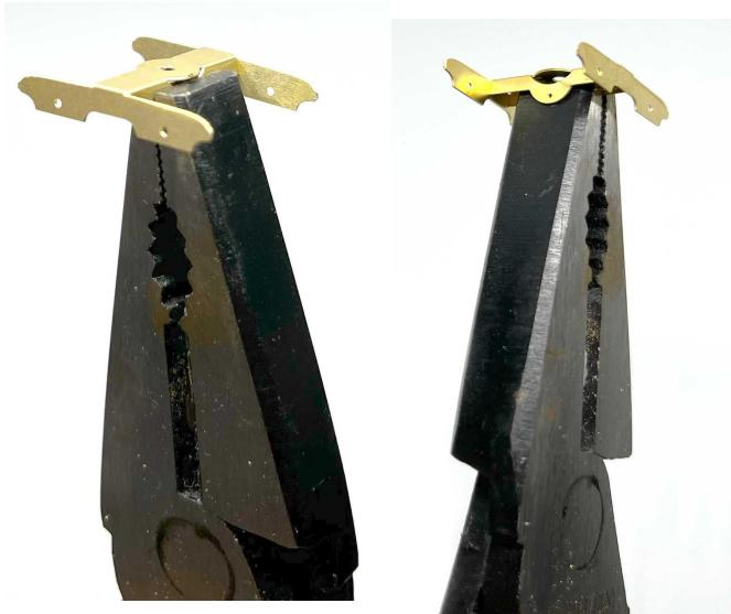
Use pliers to fold the two side wings of the centre part of the frame. You might have to overbend these parts as well, so 95 degrees. This is so the wheels don't touch it.
